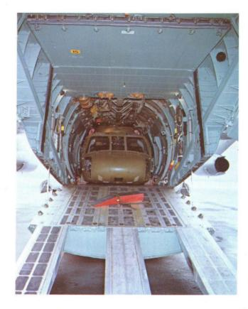
The H-60 is capable of rapid strategic deployment worldwide. It is air transportable in C-130, C-141, and C-5A aircraft. (One in a C-130, two in a C-141, and six to eight in a C-5A.)
