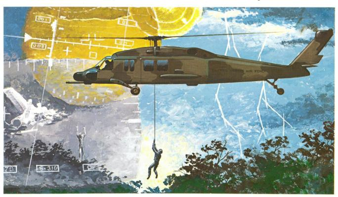
A derivative of the Army's UH-60A, the SH-60B is being developed for the Navy's LAMPS mission. In addition to different avionics, sensors, and weapons suit, the SH-60B has a higher powered engine, a larger fuel tank, an external rescue hoist, more versatile auto flight control system, a redesigned tail wheel installation and
