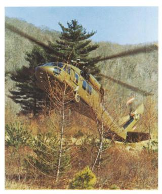
Designed to meet essential combat needs, the H-60 can hover out of ground effect at 4000 feet altitude, 95°F temperature, and even climb vertically 450 feet per minute under those conditions. In fact, under almost any temperature, altitude, or weather conditions likely to be encountered in any potential theater of operations, a combat rescue H-60 can perform the mission more effectively than any other helicopter.
